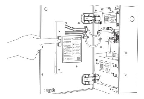
2. Press the silver tab on the dip tube connector to remove the empty tank from the fixture.
